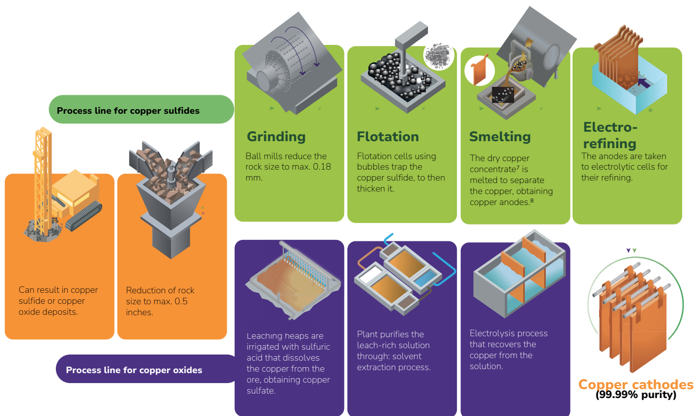
Figure 1: Copper mineral beneficiation diagram.
